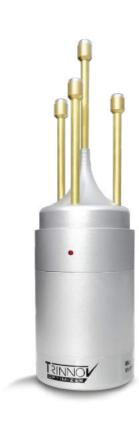
With many unique capabilities, the Optimizer's magic begins with Trinnov's iconic 3D Microphone. With 4 elements in a tetrahedral arrangement, this microphone captures sound in three dimensions, which the Optimizer uses to precisely locate the speakers, within 2° of azimuth and elevation, and 1 cm of distance. Exclusive to Trinnov, this microphone is factory calibrated to ±0.1 dB accuracy through an individual compensation file loaded onto the processor prior to the measurement.
