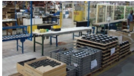
Lean Assembly Work Cells
