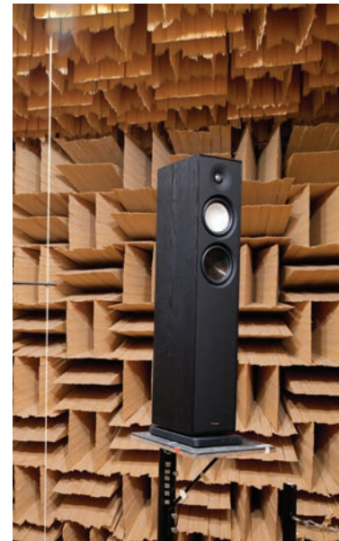
36,000 cu ft. (more than 1 million liters) Anechoic Chamber
